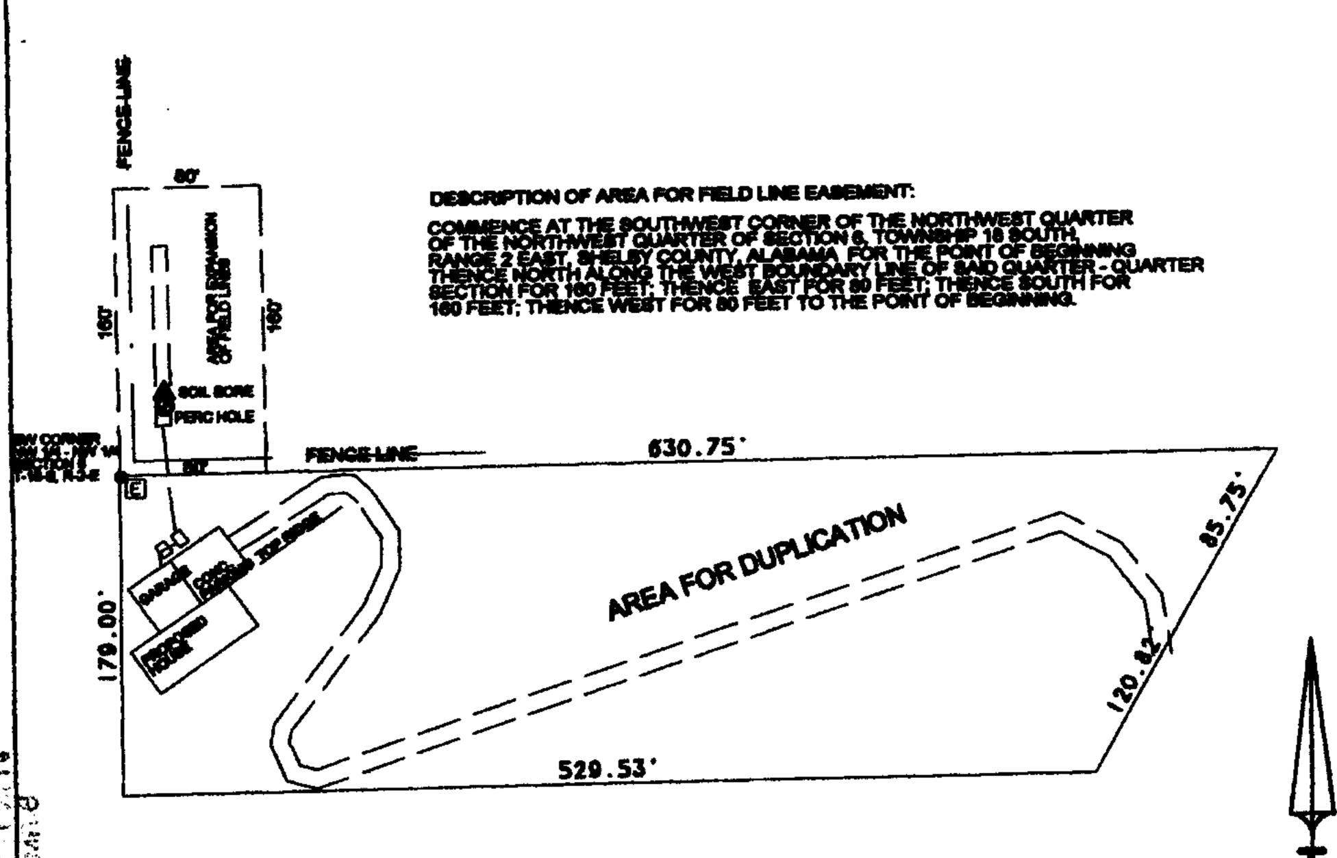
INSTALL 1000 GALLON TANK WITH 200 LINEAR FEET OF 38" WIDE TRENCH SPACED 80" ON CENTER 24" DEEP.
