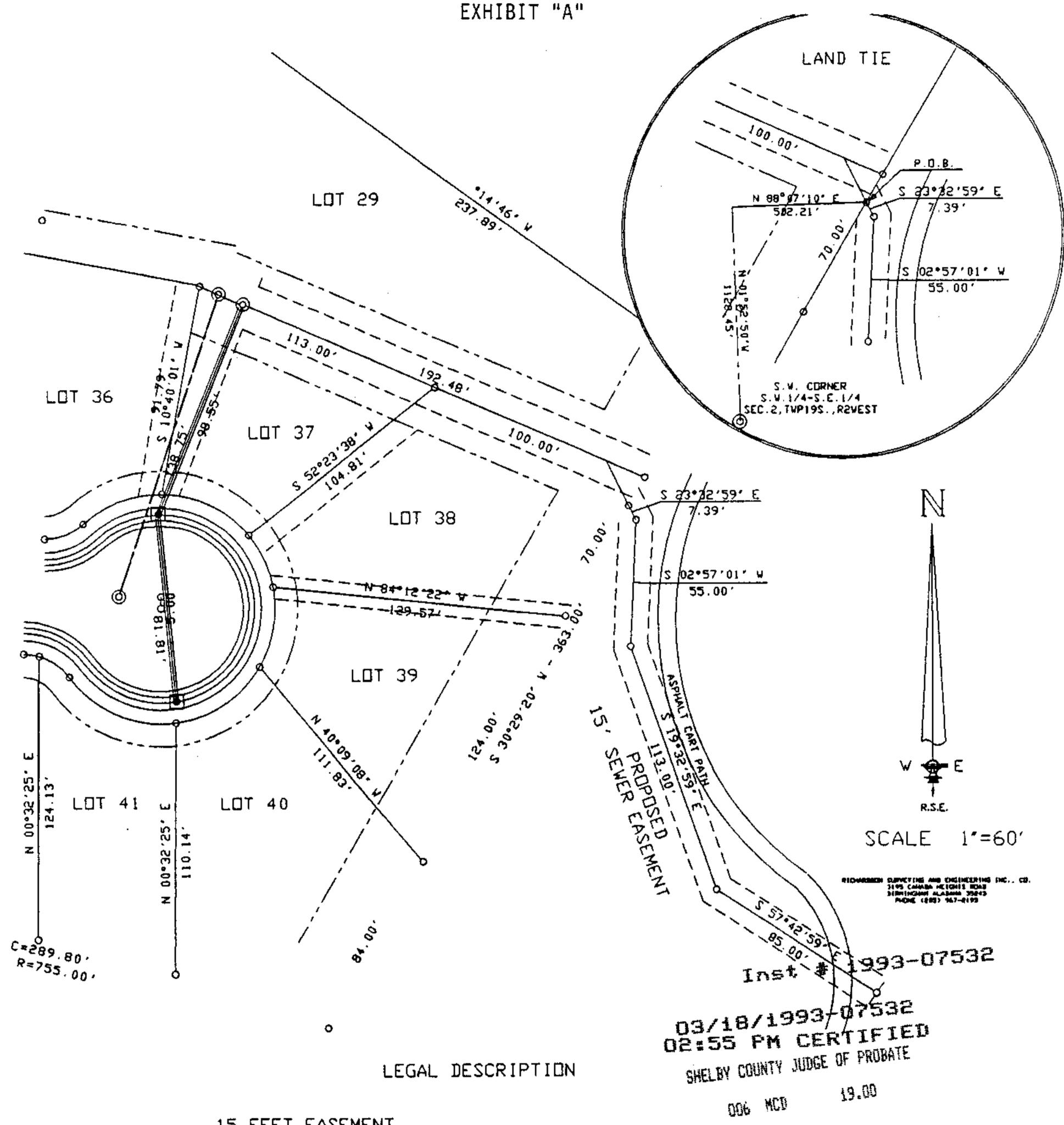
15 FEET EASEMENT FOR SANITARY SEVER PRESSURE LINE
