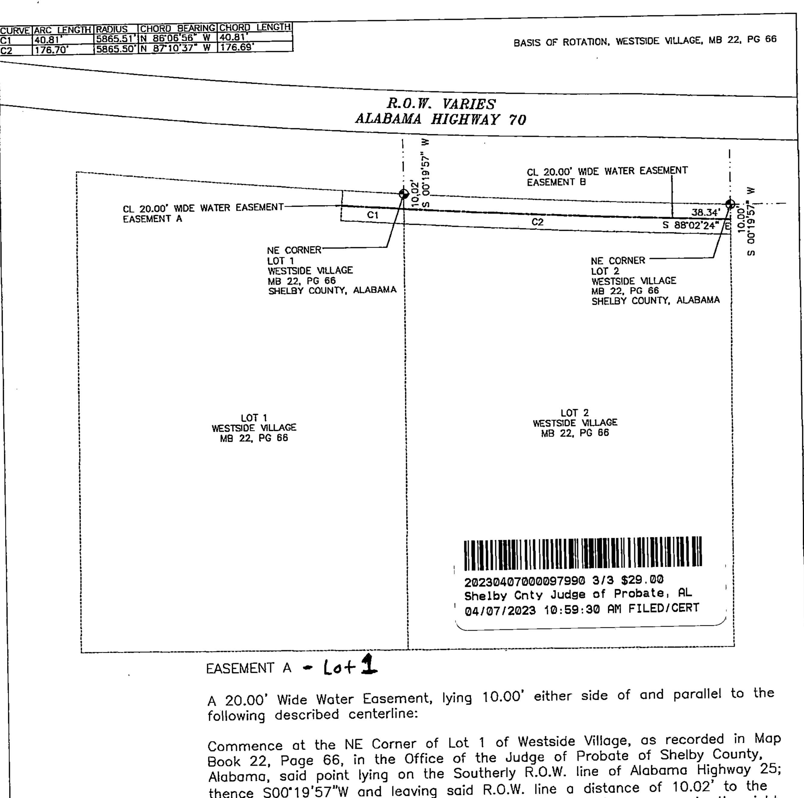
thence S00°19'57"W and leaving said R.O.W. line a distance of 10.02' to the POINT OF BEGINNING OF SAID EASEMENT; said point being a curve to the right, having a radius of 5865.51, subtended by a chord bearing N86°06'58"W, and a chord distance of 40.81'; thence along the arc of said curve for a distance of 40.81' to the POINT OF ENDING OF SAID EASEMENT.
