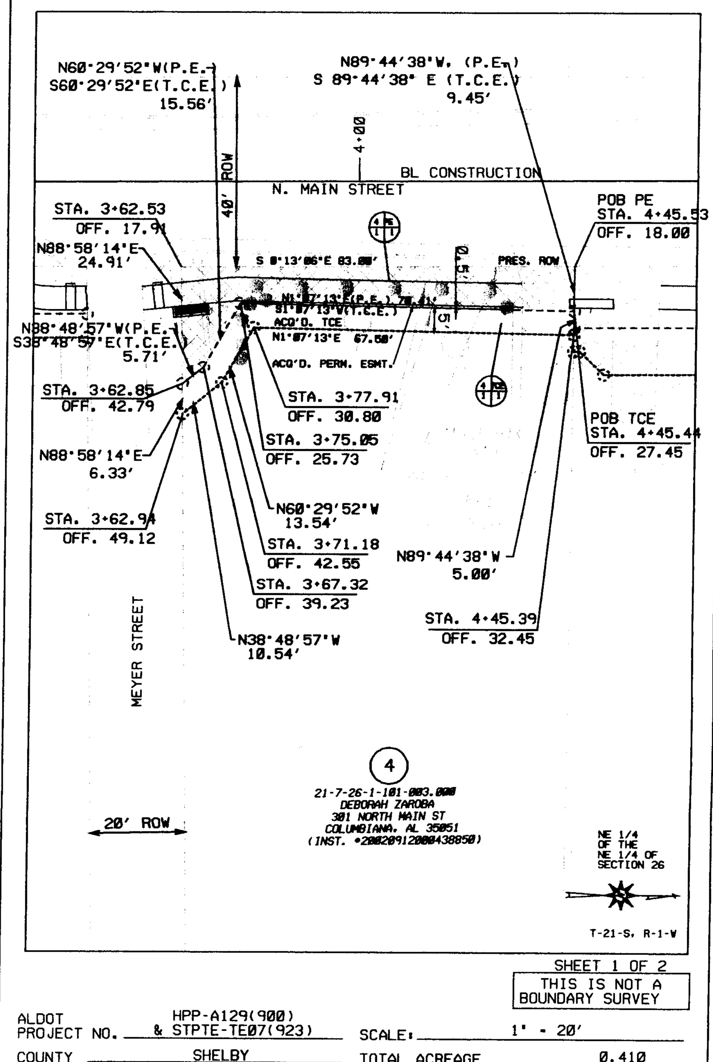
SHELBY 0.410 COUNTY TOTAL ACREAGE TRACT NO. 0.000 R.O.W. REQUIRED \_\_\_\_ DEBORAH ZAROBA 0.410 OWNER REMAINDER . 0.00PRESCRIPTIVE R/W \_\_\_\_ 0.019 REQ'D. PERMANENT EASE.\_\_\_\_ REQ'D. TEMP. CONST. EASE. 0.011
